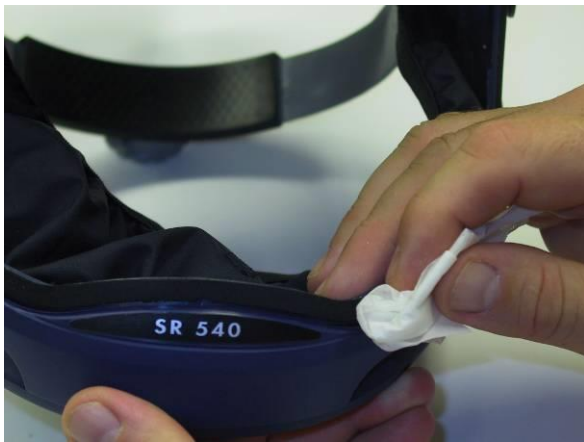
Clean around the opening seal.
