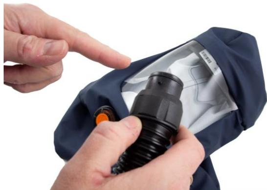
**1.2** Check that the O-ring of the hose is in place.
