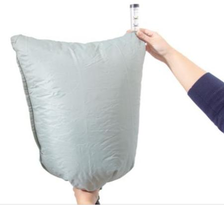
**2.2** Place the head-top in the flow meter and start the fan unit. Grip the bag to seal around the breathing hose. Grip the flow meter tube with the other hand, the tube will point upwards from the bag
