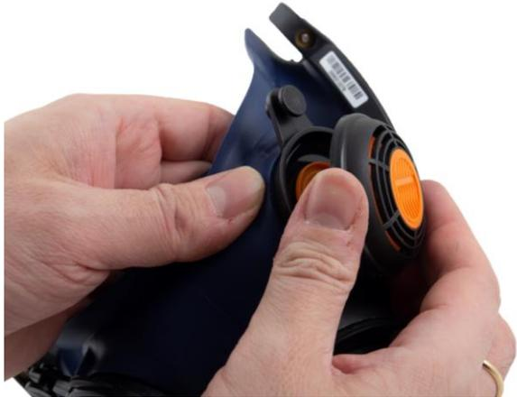
**14.1** The exhalation membranes are mounted on a fixed dowel on the inside of the valve covers on each side of the outer mask. The covers should be changed whenever the membranes are changed. Snap the valve covers off the valve seats.
