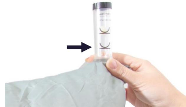
**2.2** Read the position of the ball in the tube. It should float level with or just above the marking on the tube.
