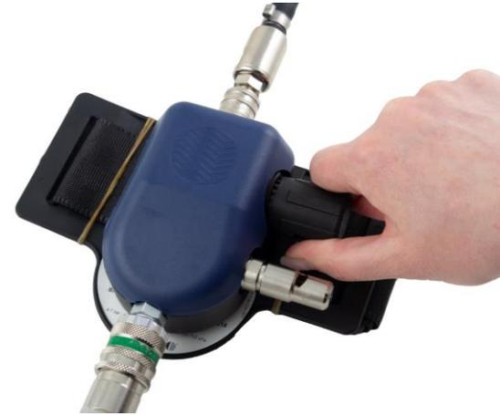
**1.6** Turn the control valve knob anti-clockwise as far as it will go, in order to throttle the air flow rate to a minimum.
