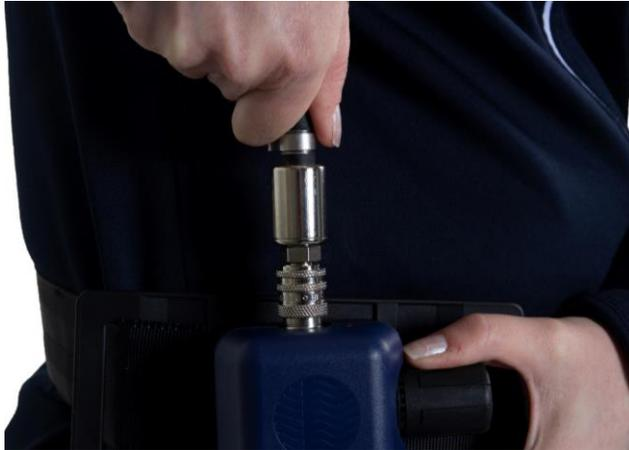
**11.1** Both couplings are of safety type and are released in two stages.
