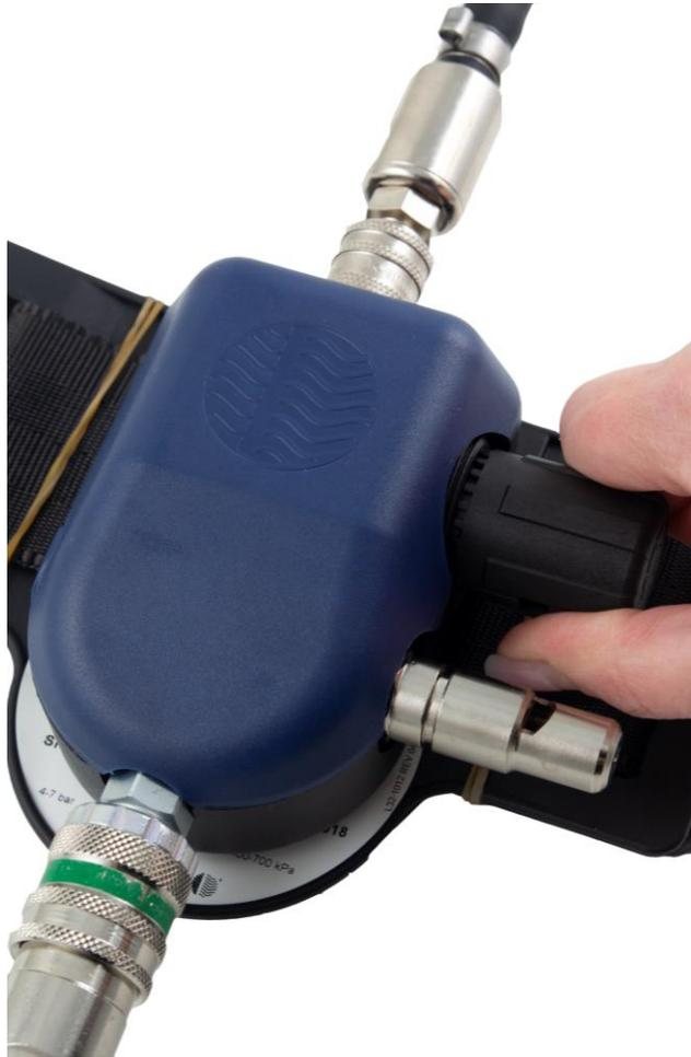
**8.1** Use the control valve knob to set the air flow rate to suit your current work intensity. In the fully closed position (turn the knob anti-clockwise), the flow is about 150 l/min. In the fully open position (turn the knob clockwise), the flow is about 320 l/min.
