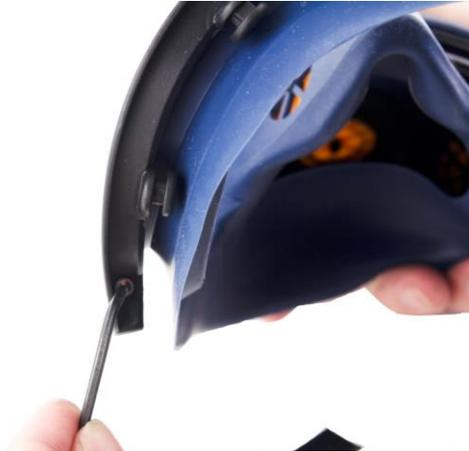
**12.1** The visor is mounted in a groove running around the visor opening of the outer mask and is held in place by one upper and one lower frame half.
