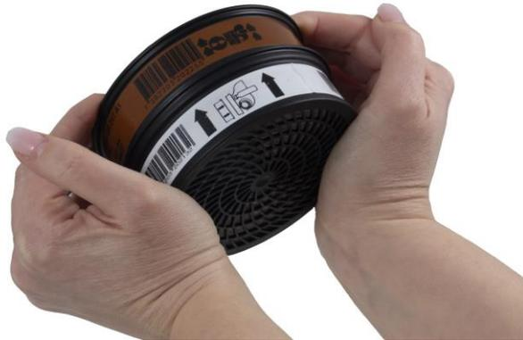
**3.1** During work in atmospheres containing both particulates and gases/vapors (such as spray painting) the particulate filter and chemical cartridge should be combined. Press the filter/cartridge together so that the arrows on the particulate filter point towards the chemical cartridge.
