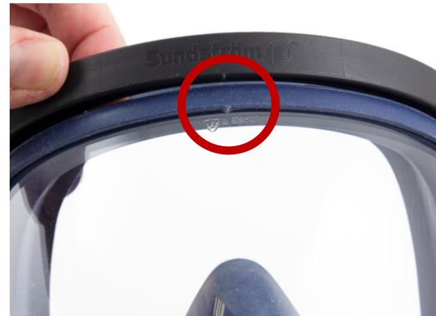
**12.6** Prise the upper frame half, making sure the centre markings are in line.
