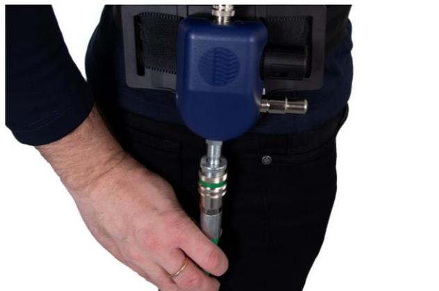
**9.2** Disconnect the compressed air hose from the control valve.
