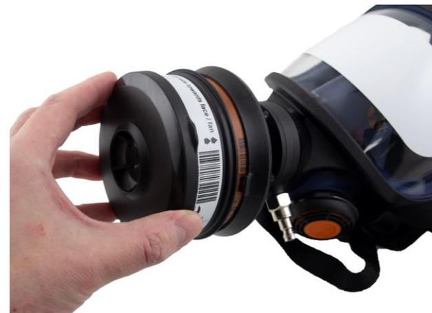
**3.4** Turn the filters into the face piece. Screw until the thread reaches the seal at the bottom of the filter connection, then another 45 degrees.
