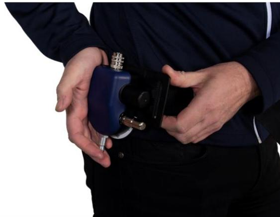
**4.2** Arrange the control valve in a way that allows easy adjustment of the flow rate and a strict watch over the breathing hose, i. e. it must not be placed on the back of the waist.
