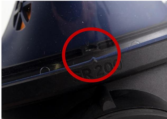
**12.4** Markings are made to show the centres of the visor, frame halves and mask. Press the new visor into the groove, making sure that the centre markings are in line. To make assembly easier, coat the slot with a soap solution or similar liquid.
