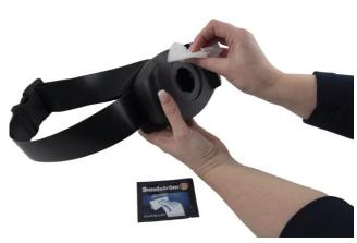
6.2 Clean the SR 905 and all parts with Sundström cleaning tissues SR 5226. If the SR 905 is heavily soiled, use a warm (up to +40 °C), mild soap solution and a soft brush, followed by rinsing with clean water and drying in air at room temperature.
