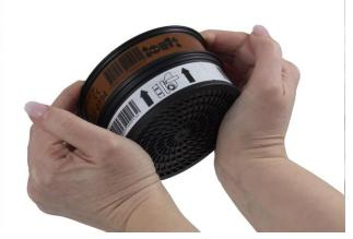
2.1 When using both gas filter and particle filter, the particle filter shall always be snapped onto the gas filter and the gas filter shall always be inserted in the filter holder. Press the filters together with your fingers placed around the outer edges of the filters until you hear a click.
