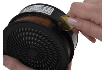
**2.3** Place a coin between the lower lip of the particle filter and the small tab molded into the side of the gas filter.
