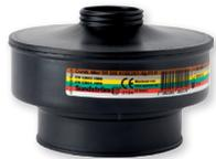
**SR 599 combination filter A1BE2K1HgP3** offers protection against organic compounds with a boiling point above +65°C, inorganic compounds and acidic gases/vapours, ammonia, mercury vapour as well as against all types of particles. It is designed for use in the SR 500 EX fan. Its maximum time of use for protection against mercury vapour is 50 hours.
